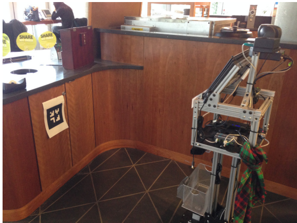
Figure 8: The CoBot checks to see if the cafe is open by conditioning on the presence of a landmark
