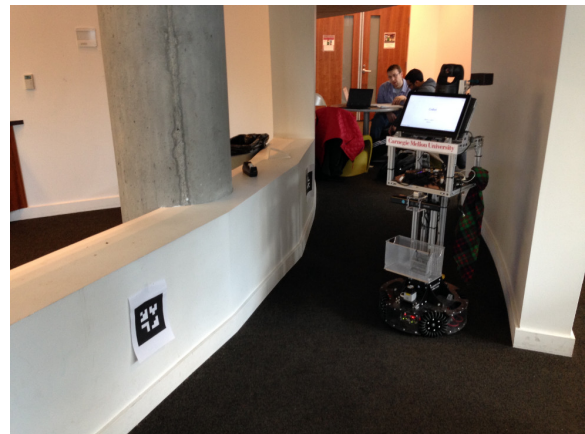
Figure 6: The CoBot navigates a bend by orienting itself with respect to several landmarks.
