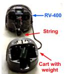
Figure 5: RV-400 tangled with a string connected to a heavy cart.
