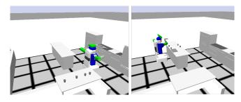
Figure 3: The "table-setting" task: moving four cups from a table to a particular arrangement on another. Left: start state; some randomization in cup and tray placement. Right: goal state; cups must be at definite positions.
