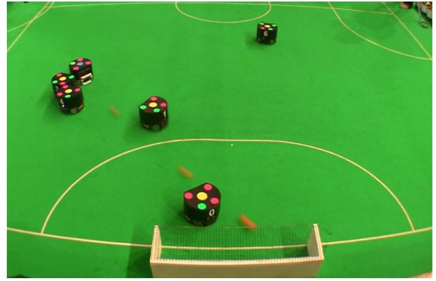
Figure 2: Goal scored by CMDragons during the quarter finals of RoboCup 2013. Accurate ball interception models of itself and of opponents allows our single robot (blue center dot) to gain control of a moving loose ball among several opponents (yellow center dots) to be able to score. (Thanks to J. Biswas [8] for the ball interception algorithm.)
