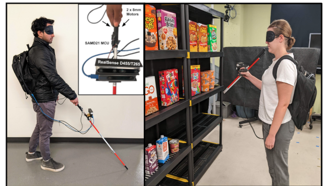
Figure 1: ShelfHelp includes a robotic cane equipped with RealSense D455 and T265 cameras. The system is powered through a laptop in a backpack. Left: The system used as a navigational device. It uses audio and haptic feedback for navigation guidance. Right: The system used as a manipulation device. It uses audio for manipulation guidance.
